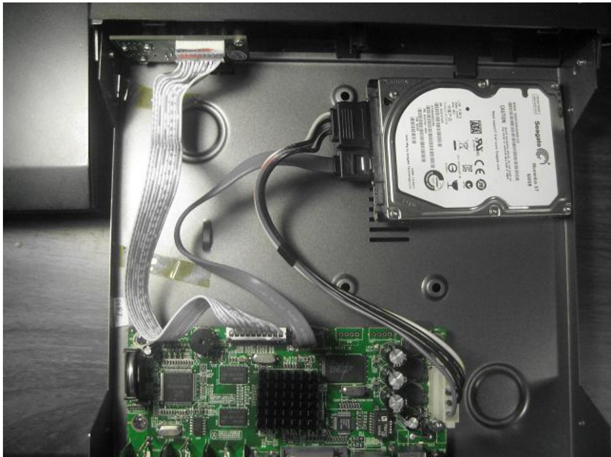
Figure 3. Installation of SATA Hard driver
